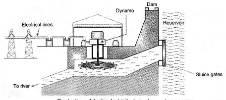
Production of hydroelectricity by using water energy
